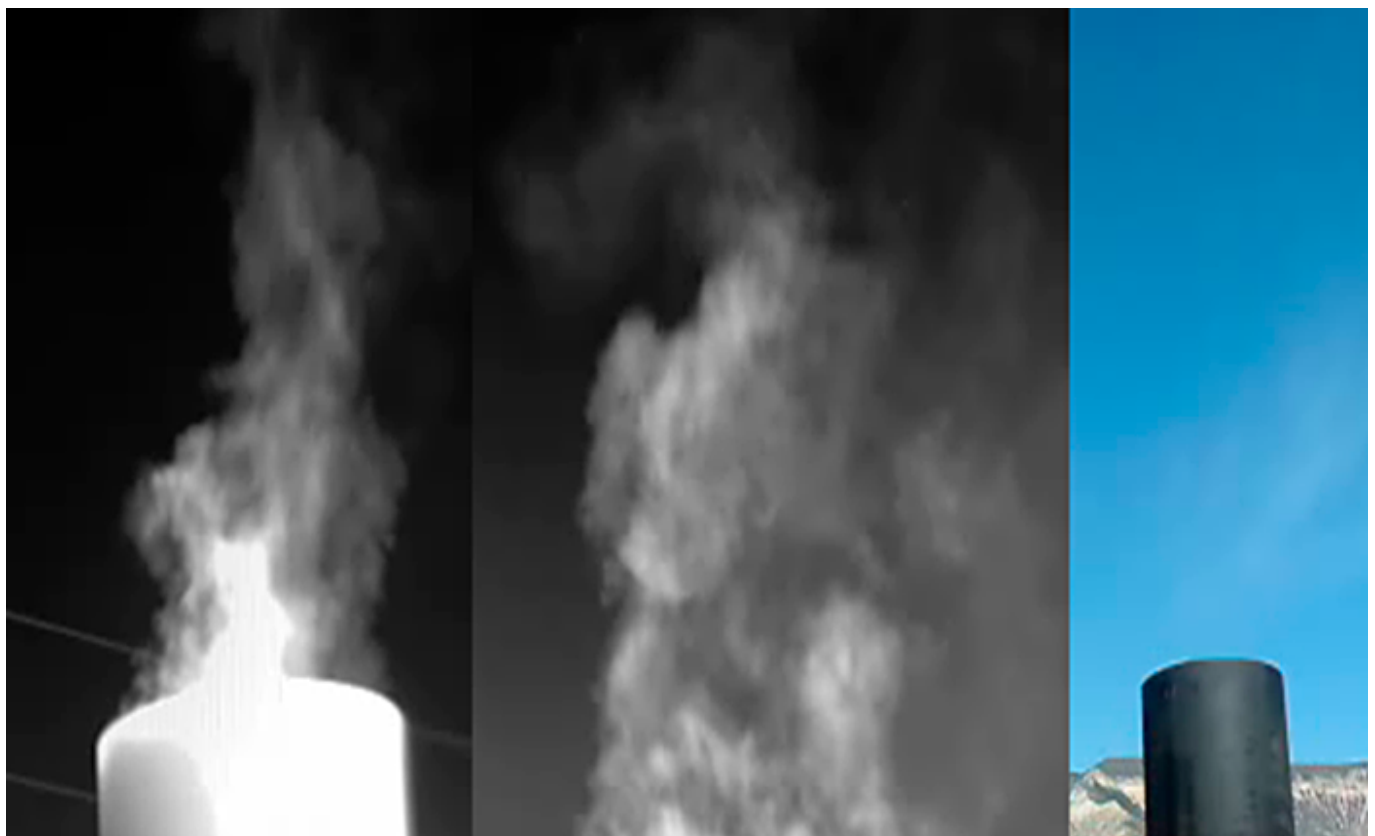
Figure 63. Potentially unburned hydrocarbons observed from an enclosed flare/combustor. Pan IR camera to move white hot stacks out of viewfinder to check if plume is hanging together. Source: Provided by USEPA.
