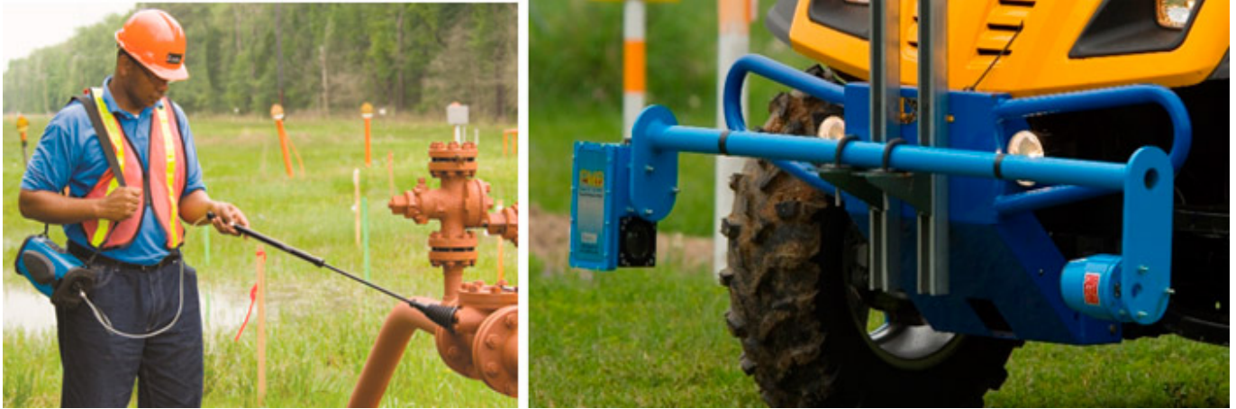
Figure 30. Example of Etalon-based instruments used for methane leak detection.
