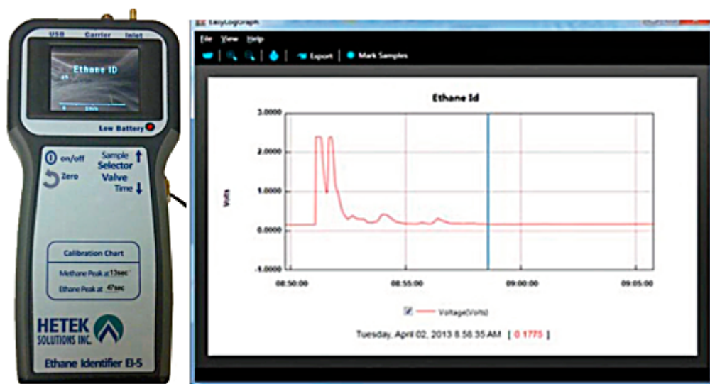
Figure 10. Example of a portable ethane identifier for discriminating natural gas containing ethane.
