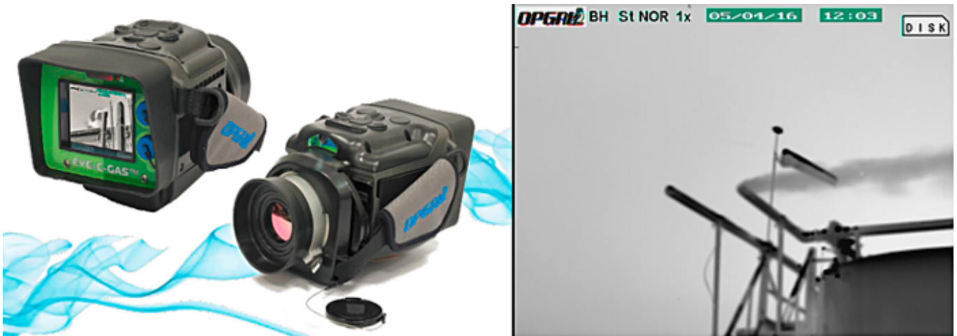
Figure 33. OGI Camera and image of a leak through a relief valve.
