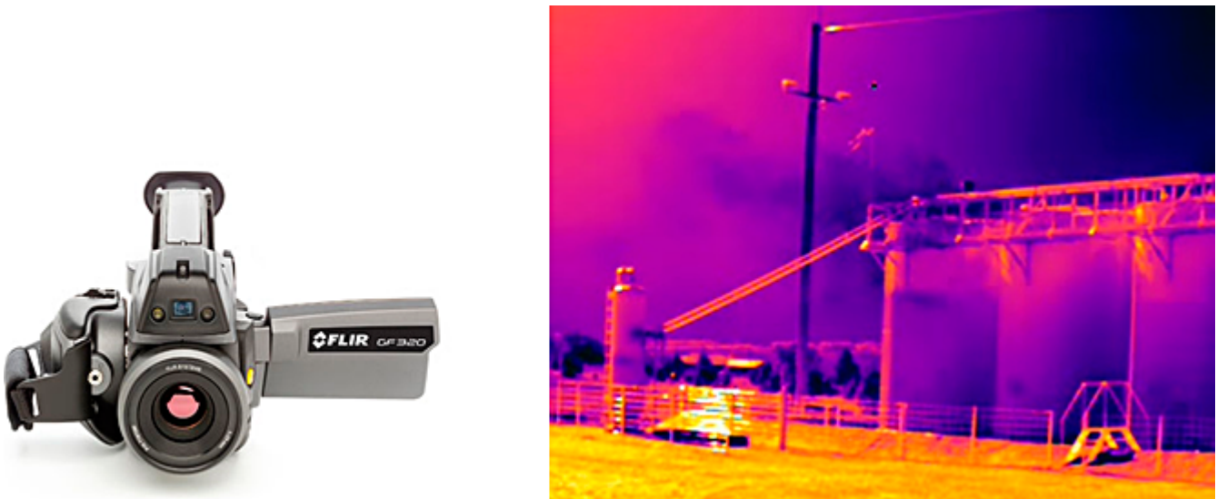
Figure 34. Optical gas imaging camera and image of a leak.
